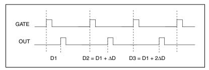
Figure 7-28. Pulse Generation for ETS
